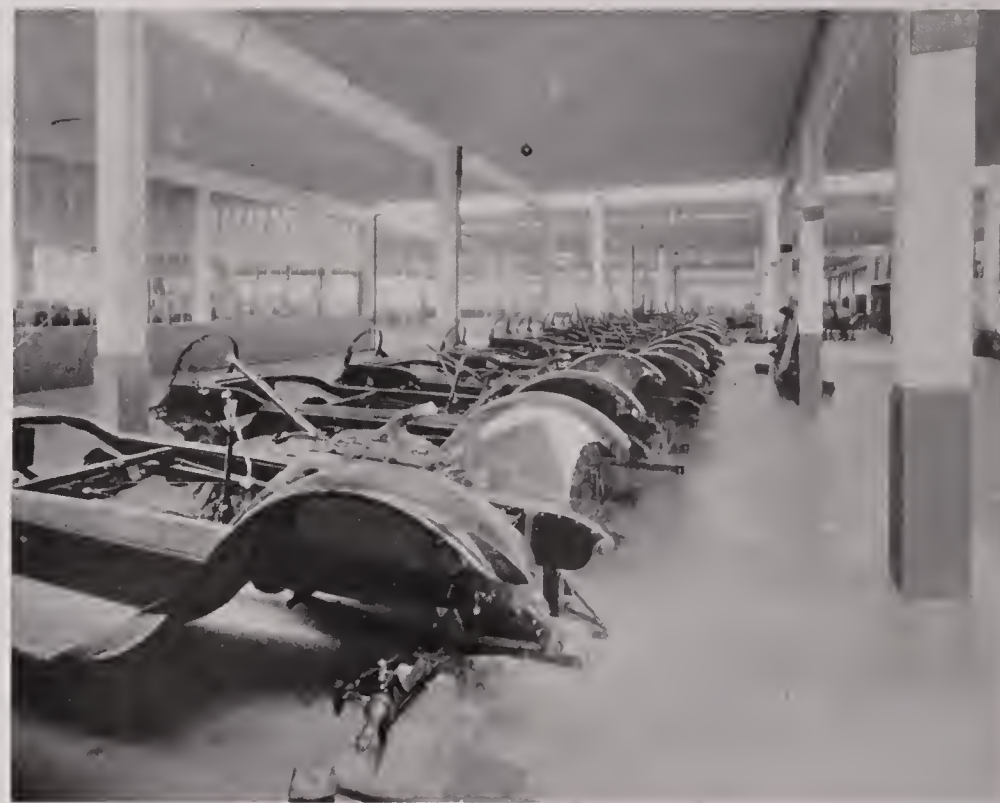
CHASSIS READY FOR FINAL ASSEMBLIES
